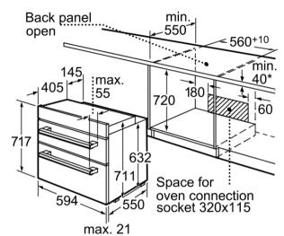
\* For installation under an induction hob min. 50 mm measurements in mm
