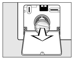
Remove the drain filter completely.
