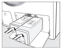
Push the UltraPhase 1 cartridge into compartment ① and the UltraPhase 2 cartridge into compartment ②, until they lock into position.
