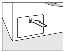
Press the drain pump access panel.
