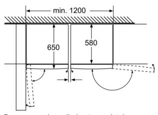
Drawers can be pulled out completely if the appliance is placed directly on a wall.
