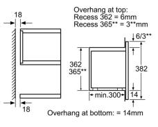
Measurements in mm
