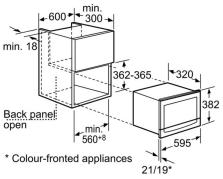
Measurements in mm
