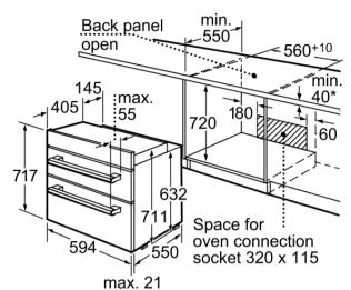
\* For installation under an induction hob min. 50 mm
